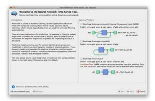
Network diagrams shown in the Neural Time Series Tool, Neural Training Tool, and with the view(net) command, have been improved to show tap delay lines in front of weights, the sizes of inputs, layers and outputs, and the time relationship of inputs and outputs. Open loop feedback outputs and inputs are indicated with matching tab and indents in their respective blocks.
