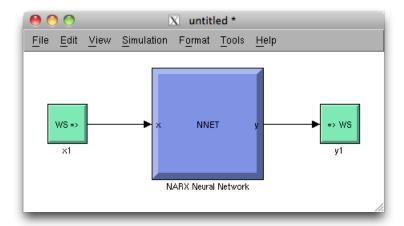
Simulink neural network blocks now allow initial conditions for input and layer delays to be set directly by double-clicking the neural network block. setsiminit and getsiminit provide command-line control for setting and getting input and layer delays for a neural network Simulink block.
